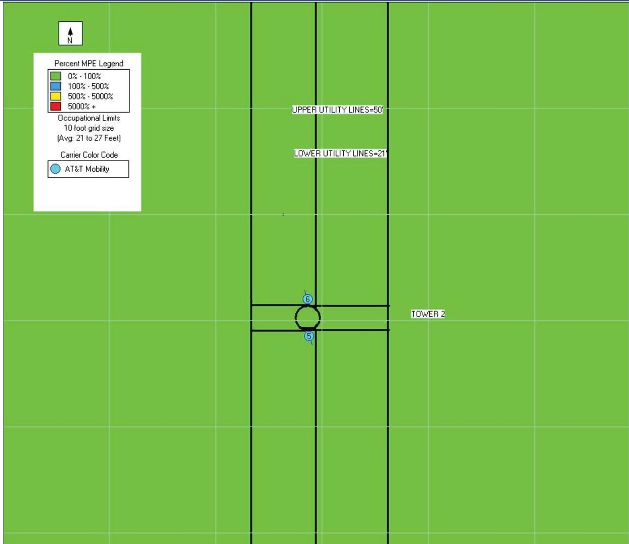
The reference plane for the plot is the 21' utility line level-Tower 2
