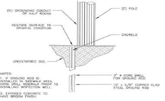
**POLE GROUNDING ROD** SCALE: NTS 4
