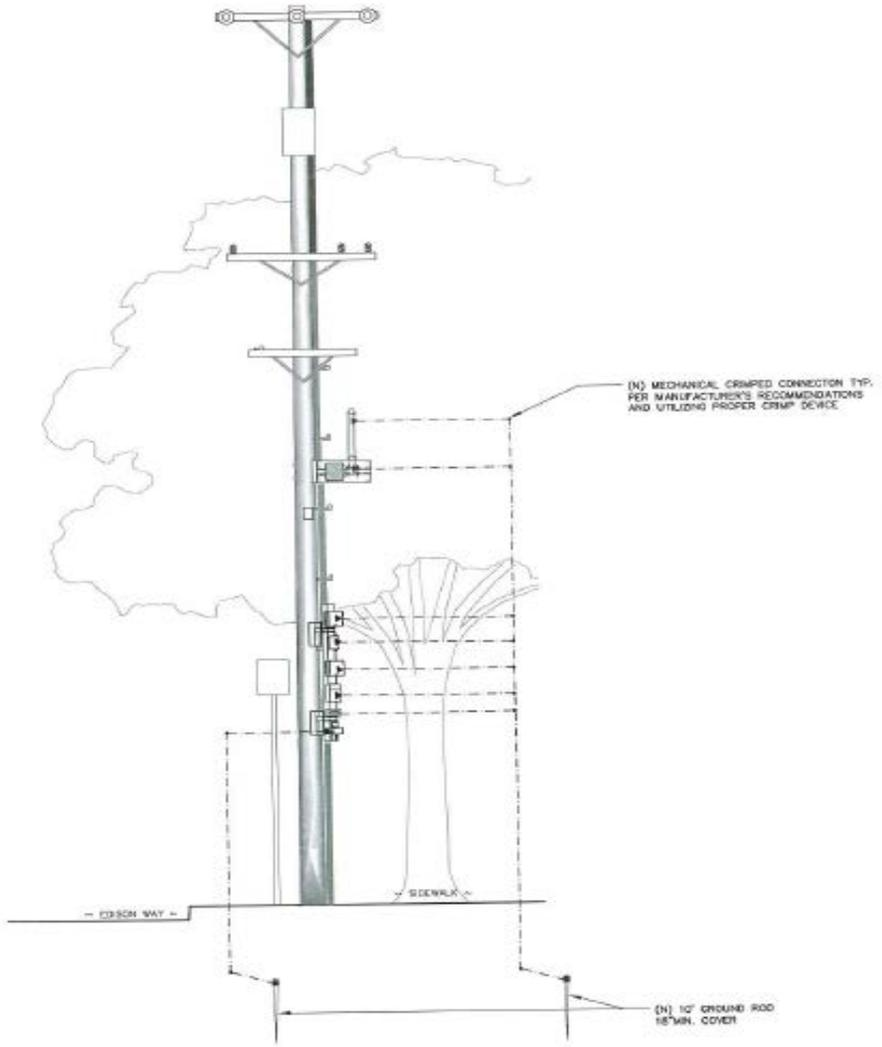
7 POLE GROUNDING DIAGRAM SCALE: 3/8" = 1'-0"
