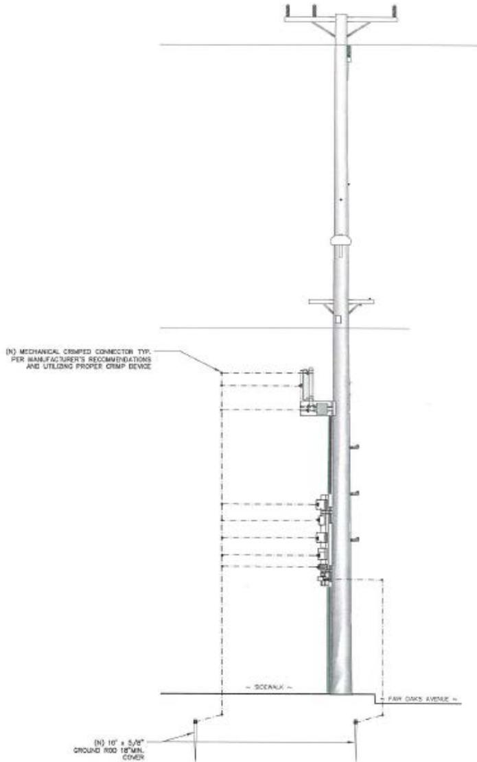
7 POLE GROUNDING DIAGRAM SCALE 3/8" = 1'-0"
