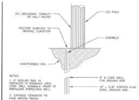
POLE GROUNDING ROD SCALE: 3/8" = 1'-0"
