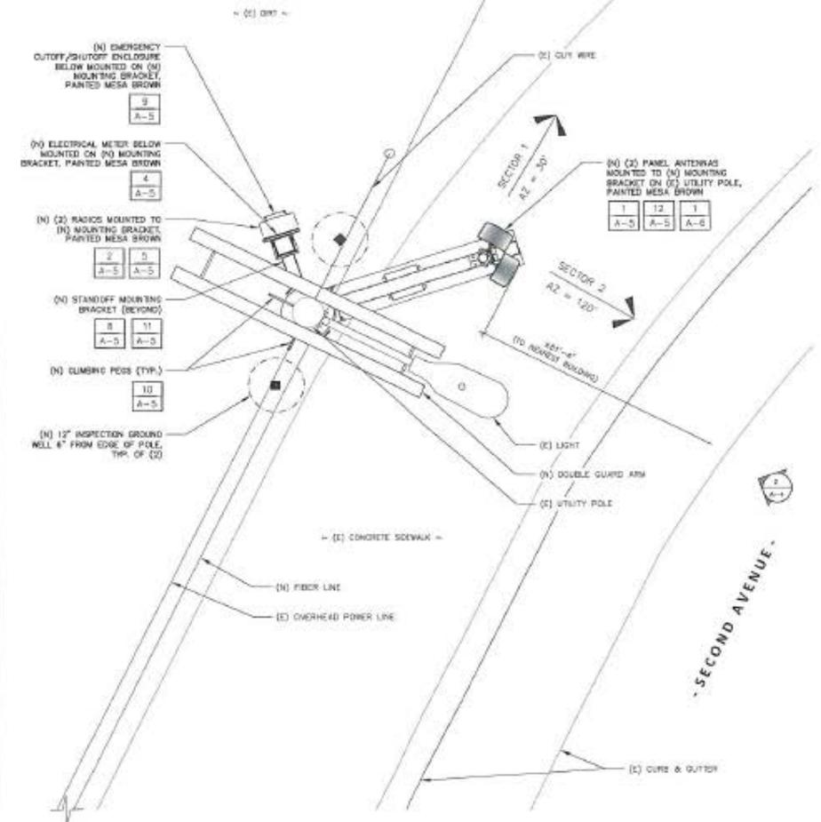
**2** PROPOSED EQUIPMENT AND ANTENNA PLAN
