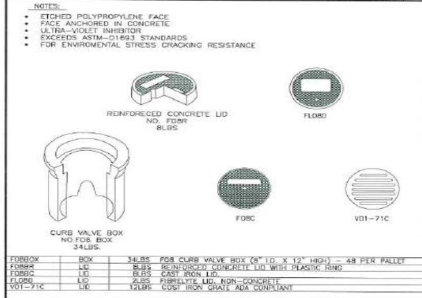
**F08 BOX GROUND WELL DETAIL** SCALE: NTS 5
