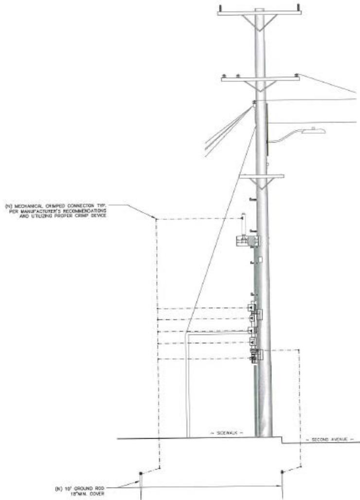
7 POLE GROUNDING DIAGRAM SCALE: 3/8" = 1'-0"
